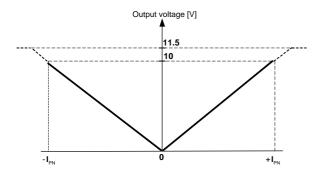
Note: 1) The performance specified in the datasheet is valid within the 0-10 V DC output range only.
